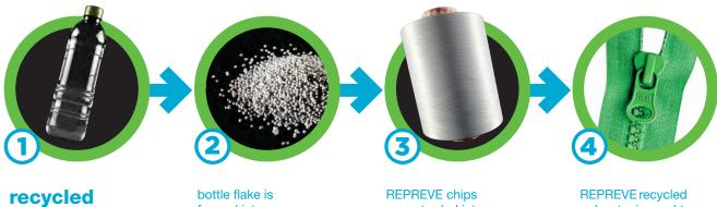
recycled bottles are collected and flaked bottle flake is formed into REPREVE chips
